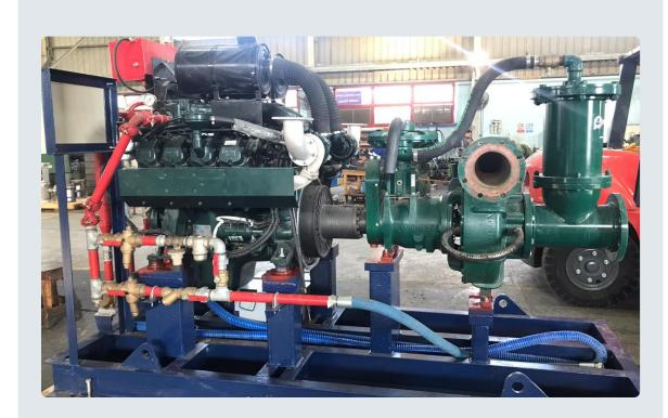
Shotec has finalized the Engineering & packaging for Self-Priming Fire Pump package to Petroleum Pipe Line Co. (PPC). The pump manufacture is Pioneer and derived by DOOSAN Diesel Engine (555HP).
